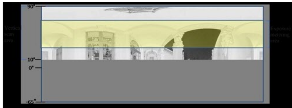
Figure 5-22 Exposure metering area for a limited vertical scan area set to e.g., 10^\circ to 90^\circ
